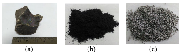
Figure 1. Starting material: (a) ferromanganese lump, (b) ferromanganese powder, and (c) aluminium powder
