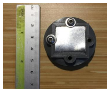
Figure 1. Sample being held by a 3D printed sample holder
