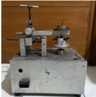
Figure 2. Pin-on-disk wear test machine
