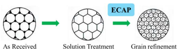
Figure 9. Grain refinement process on pure magnesium through solution treatment.
