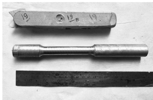
Figure 1. Specimen for tensile and impact testing
