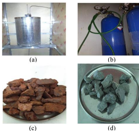
Gambar 1. (a) Vertical tube furnace , (b) Gas produser, (c) Bijih besi, (d) Besi spons
