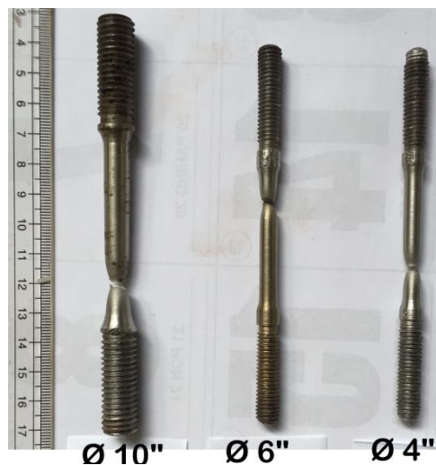
Figure 3. The three broken tensile test specimens after being tested at 300 °C
