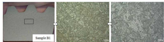
Figure 31. Microstructures obtained from sample B1 at location indicated by rectangular grid
