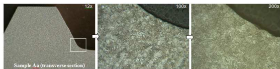
Figure 17. Microstructures obtained from sample Aa at a spline tooth root indicated by rectangular grid
