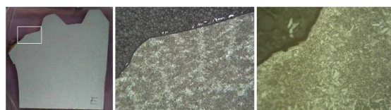
Figure 23. Microstructures obtained from sample A1 at fatigue crack initiation site indicated by rectangular grid
