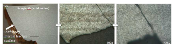
Figure 21. Microstructures obtained from sample Ab at an area located in the shaft body internal fracture surface indicated by rectangular grid
