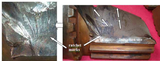
Figure 10. Close up view of the surface fracture area, showing fatigue crack growth in two different directions. Under the splines (engagement) area, the fatigue crack grew in a combined direction of transverse and radial, while outside the splines (engagement) area the fatigue crack grew approximately 45° to the shaft axis and later turned in radial direction to form a “whirlpool” crack pattern along the body shaft circumference prior to form an overload final fracture typical of cup like shape
