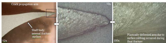
Figure 27. Microstructures obtained from sample A2 at location around the shaft body final fracture area indicated by rectangular grid
