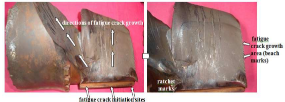
Figure 9. Close up view of the fatigue fracture surface exhibits crack initiation sites along the spline root having with some ratchet marks of a highly stressed area and the crack propagation area indicated by beach marks formation. The final fracture area is not seen in this figure as it was formed on the other side of the body shaft within the cup fracture portion
