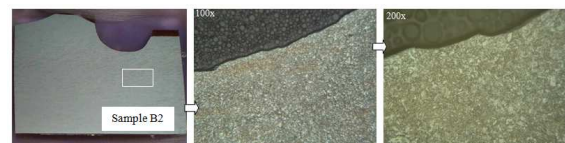
Figure 32. Microstructures obtained from sample B2 at location around the groove as indicated by rectangular grid
