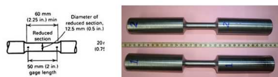
Figure 14. Drawing and dimension of tensile specimen used in failure analysis. The two tensile test specimens were made from the unbroken quill shaft B
