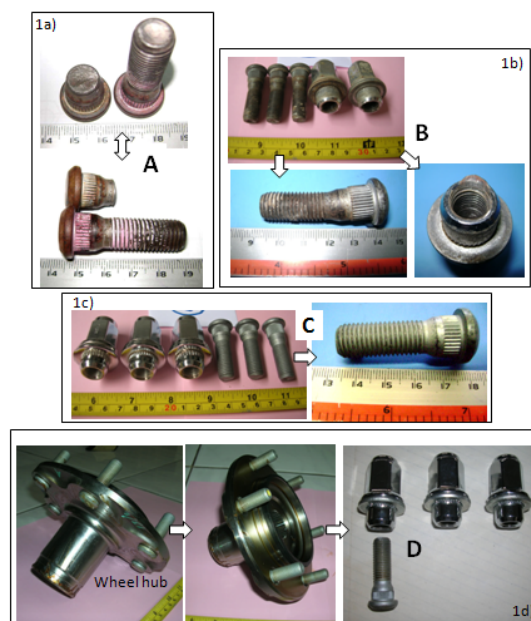
Figure 1. The as received damaged and undamaged wheel studs and nuts for metallurgical assessment. (a) Studs A recovered from the well-known brand name LV 4x4; (b) Studs and nuts B also recovered from the same brand name LV as studs A, but from different vehicle; (c) Studs C represent a non OEM; and (d) Studs D represent the OEM of the same brand name LV as studs A and studs B
