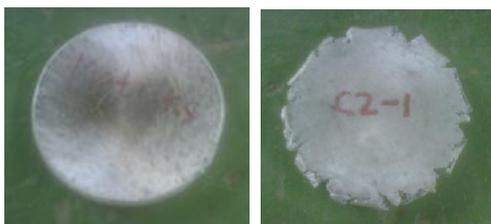
**Gambar 5.** (a) Material matriks; (b) komposit matrik paduan Al-6,2%Mg/ $Al_2O_{3(p)}$  hasil tempa
