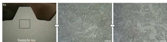
Figure 18. Microstructures obtained from sample Aa at location indicated by rectangular grid
