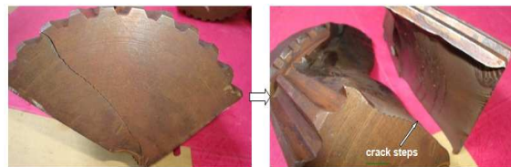
Figure 8. Cracks path direction and position located under the splines (the engagement) area and within the body shaft (outside the engagement area) observed from different views. Several crack steps were formed on the edge indicating of fatigue crack growth
