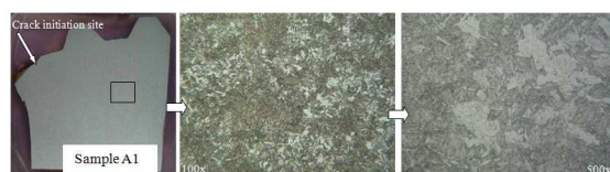
Figure 24. Microstructures obtained from sample A1 at location indicated by rectangular grid
