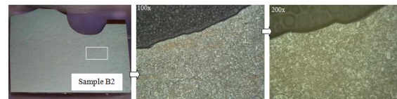
Figure 32. Microstructures obtained from sample B2 at location around the groove as indicated by rectangular grid
