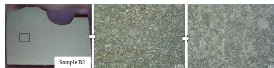
Figure 33. Microstructures obtained from sample B2 at location around the shaft body as indicated by rectangular grid
