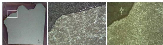
Figure 23. Microstructures obtained from sample A1 at fatigue crack initiation site indicated by rectangular grid
