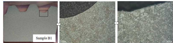
Figure 30. Microstructures obtained from sample B1 located around the spline tooth as indicated by rectangular grid
