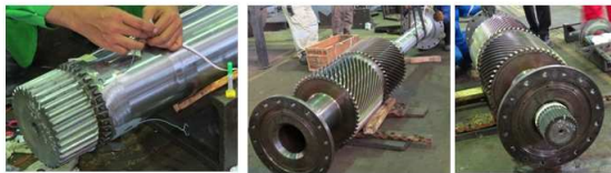
Figure 3. A new quill shaft and its installation into the pinion second reduction assembly
