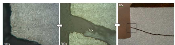
Figure 20. Microstructures obtained from sample Ab at a cracked spline tooth indicated by rectangular grid
