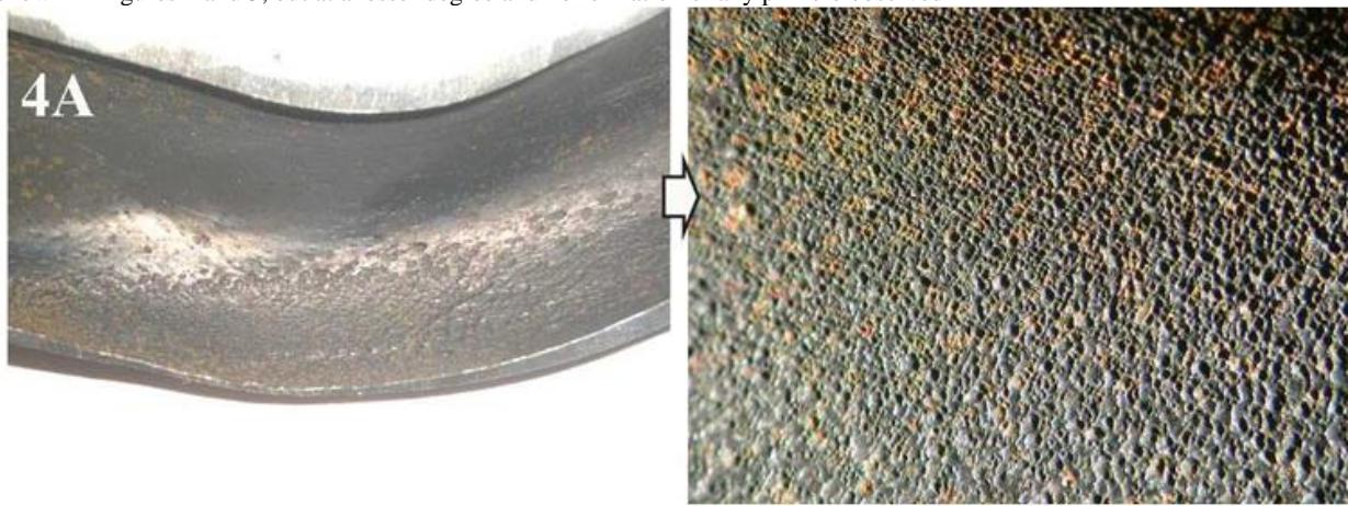
Figure 7. The elbow tube 4A showing the lowest degree of cavitation-erosion damage due to the largest its bend radius
