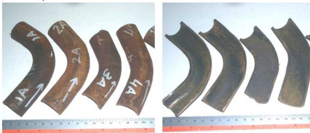
Figure 3. The four elbow tubes (1A to 4A) divided into two parts for the preparation of laboratory test samples
