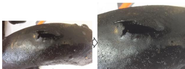
Figure 2. Close up view of the burst return bend, showing some excessive thinning or metal loss occurred around its burst and bulging area on the outer bend external surface
