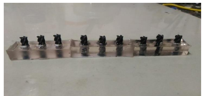
Gambar 3. Sampel cutter end mill uji SEM
