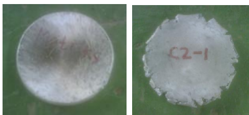
Gambar 5. (a) Material matriks; (b) komposit matrik paduan Al-6,2%Mg/ Al_2O_{3(p)} hasil tempa
