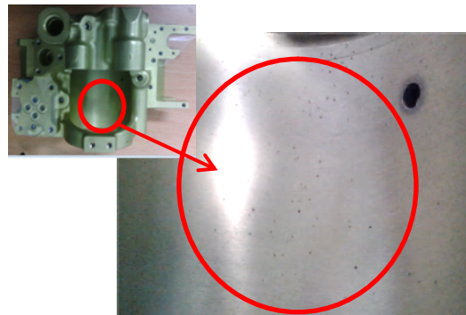
Figure 1. As received machined aileron block that revealed several pits on some of its main bore area
