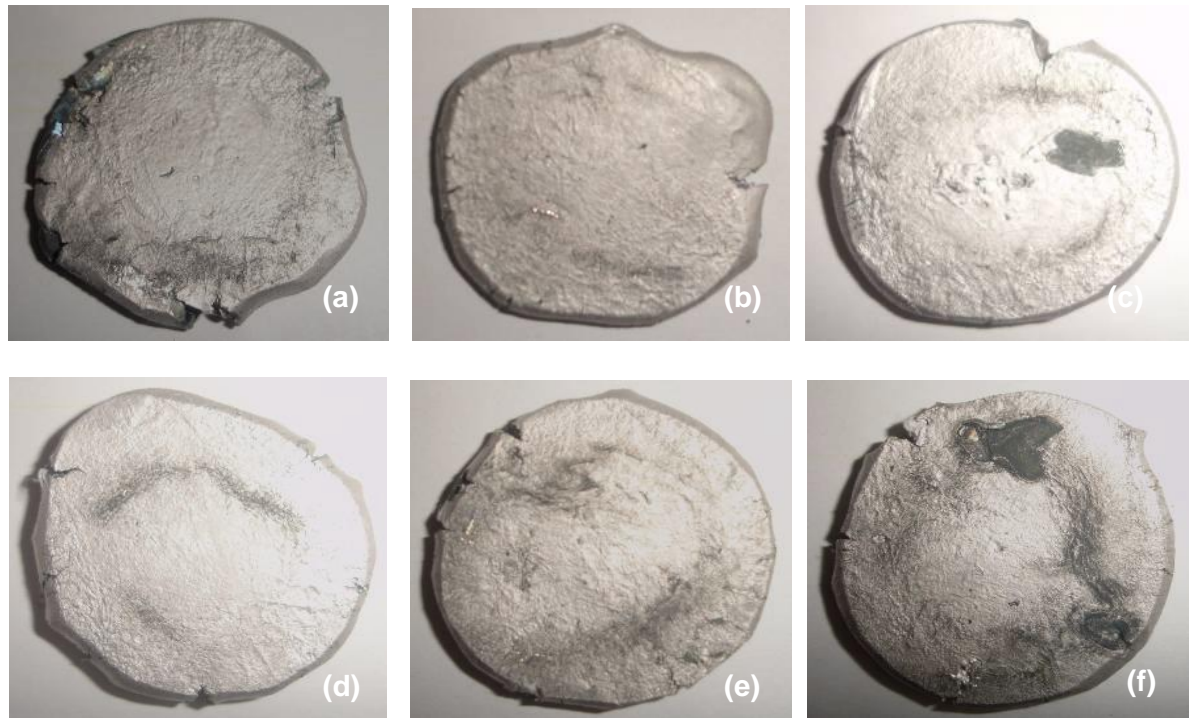
Gambar 4. Ingot paduan hasil tempa pada T= 1250\text{ }^{\circ}\text{C} : (a) Co-35Cr-5Mo; (b) Co-35Cr-5Mo-0,2Mn; (c) Co-35Cr-5Mo-0,4Mn; (d) Co-35Cr-5Mo-0,6Mn; (e) Co-35Cr-5Mo-0,8Mn dan (f) Co-35Cr-5Mo-1Mn
